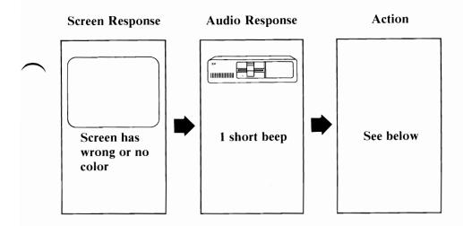
If you are using a TV as your display, verify that the color is correct by disconnecting your TV from the unit and operating the TV normally. Also, ensure your TV is compatible with the NTSC standard. If you have an IBM Color Display, go to Test 9000.
