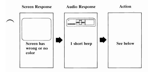
If you are using a TV as your display, verify that the color is correct by disconnecting your TV from the unit and operating the TV normally. Also, ensure your TV is compatible with NTSC standard. If you have an IBM Color Display, go to Test 9000.
