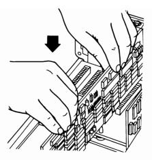
When inserting an option adapter into the system board, grasp it by its top edge or upper corners.
