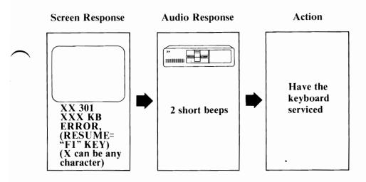
**Note:** Ensure the keyboard is connected correctly and check for any objects or foreign material on the keyboard. If error 301 still appears after the keyboard has been serviced, have the system unit serviced.
