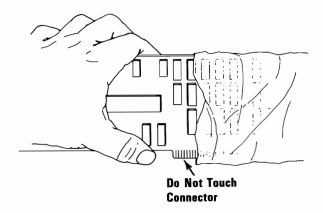
Carefully remove the option from its anti-static bag. Be sure to handle circuit boards by the edges only and do not touch the component pins or solder joints. Grasp diskette drives and fixed disk drives by their frames to avoid touching the circuit board. Memory chips should be held by their narrow ends only, not by their pins.
