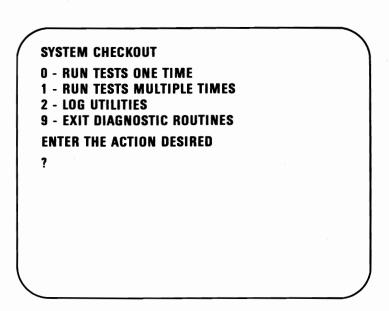
The diagnostic programs have successfully loaded. Continue with the tests on the following pages to perform a complete system checkout.
