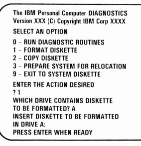
YES - Remove the Diagnostics diskette from drive A, insert a blank diskette push the load lever down.
