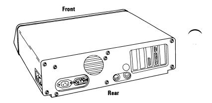
Connect the keyboard cable to the system unit.
