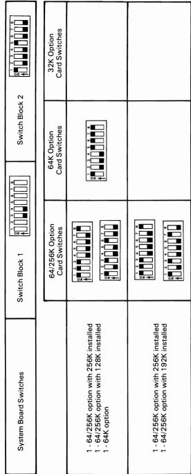
512K Total Memory 448K + 64K on System Board 544K Total Memory 480K + 64K on System Board
