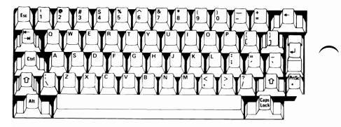
Key positions in the typewriter area are much like those of a standard typewriter. Some additional keys, however, perform control functions.
