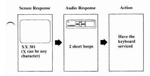
**Note:** Ensure the keyboard is connected correctly and check for any objects or foreign material on the keyboard. If error 301 still appears after the keyboard has been serviced, have the system unit serviced.
