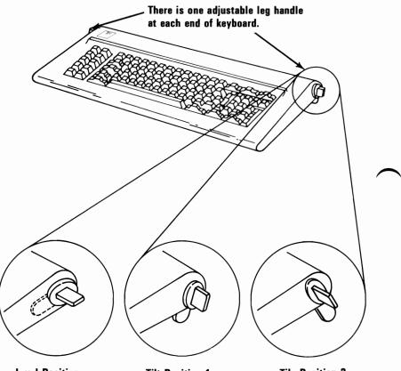
Level Position Firmly push in the adjustable leg handles and turn. Tilt Position 1 This position may not be available on your keyboard. Tile Position 2 Firmly push in the adjustable leg handles and turn.
