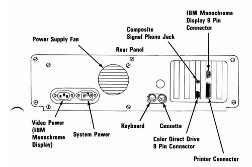
If you have an expansion unit, connect it to your IBM Personal Computer as shown below. Connect the expansion unit's power cord to the expansion unit, then to the wall outlet.
