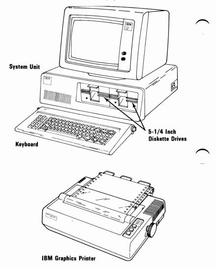
This example shows the system unit, keyboard, IBM Monochrome Display, and IBM Graphics Printer. Two 5-1/4 inch diskette drive units are used to store programs and data. Hard-copy output is provided with the IBM Graphics Printer.
