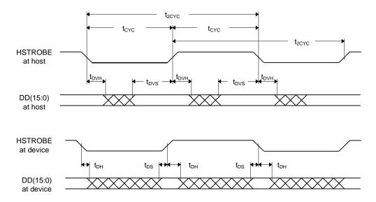
Figure 5 - 10 Sustained Ultra DMA Data Out Burst
