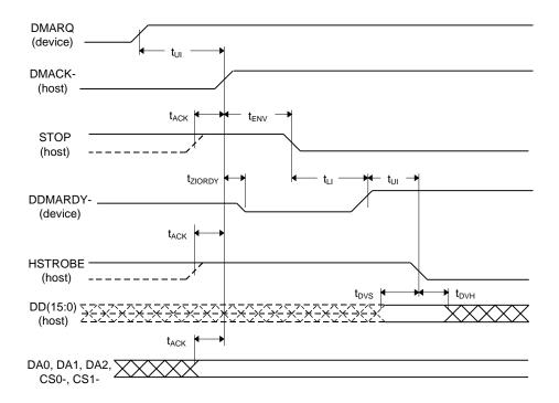
Figure 5 - 9 Initiating an Ultra DMA Data Out Burst
