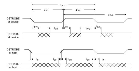
Figure 5 - 5 Sustained Ultra DMA Data In Burst
