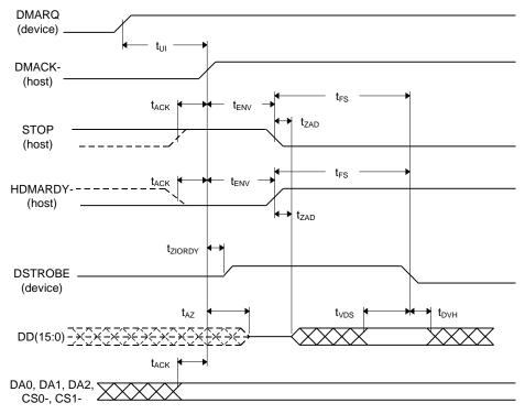
Figure 5 - 4 Initiating an Ultra DMA Data In Burst
