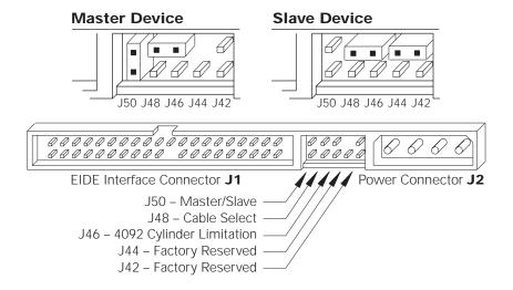
Figure 4 - 4 Master/Slave Jumper Detail
