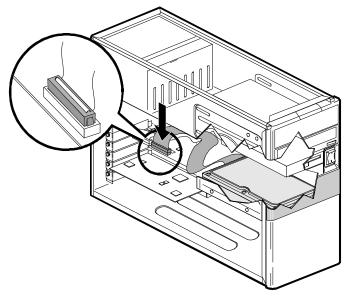
Figure 4 - 9 System Interface Card Cabling
