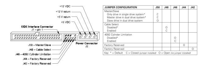
Figure 2-1 PCBA Jumper Location and Configuration
