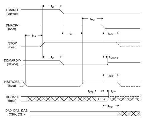
Figure 5 - 12 Host Terminating an Ultra DMA Data Out Burst
