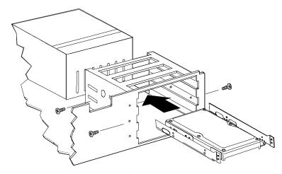
Figure 4 - 6 5.25-inch Installation
