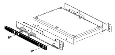
Figure 4 - 5 5.25-inch Mounting Brackets/Slider Rails
