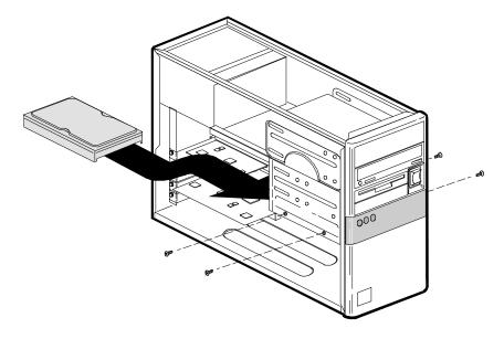
Figure 4 - 7 3.5-inch Installation
