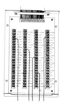
**Note:** Make sure that you do not pinch the wires when you place the cover on the distribution panel.
